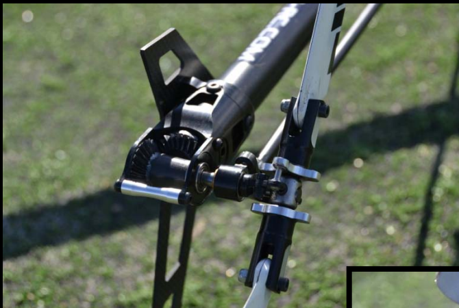
≡View of the tail rotor and the bearings inside
