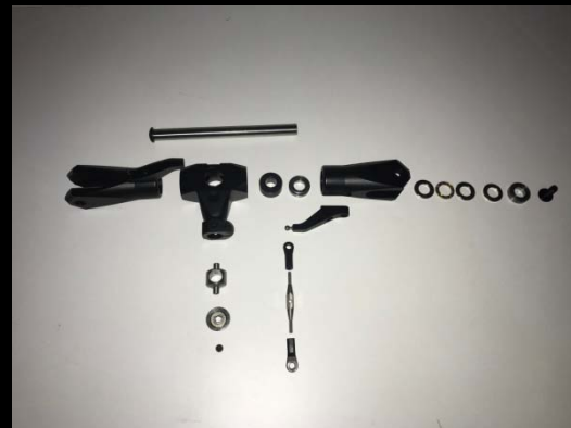
≡ Details of ball bearings and another pieces which compose the main rotor
