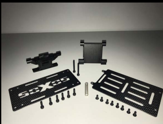
≡ ESC tray was modified to use large ESC's
